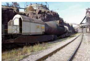
Torpedo transporting iron from the blast-furnace to the steelworks. SSAB Tunnplåt AB, Luleå, Sweden. Photograph: Stig-Göran Nilsson (2002)
